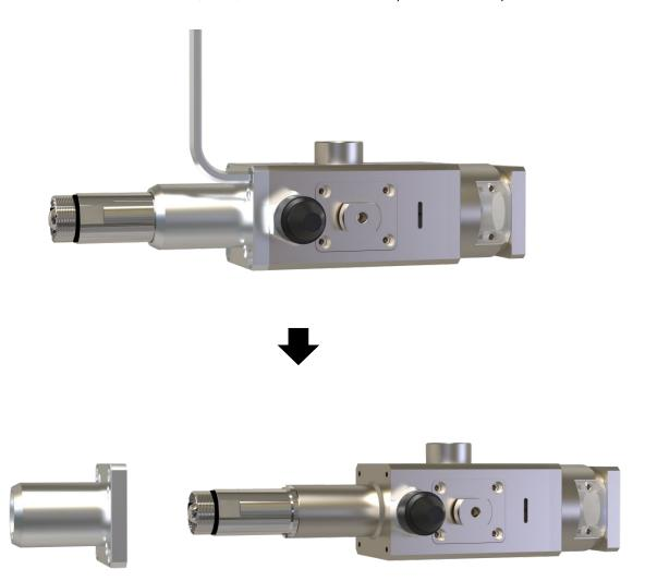
5) Turn the four wrench bolts(M3x12) counterclockwise to separate motor block.
