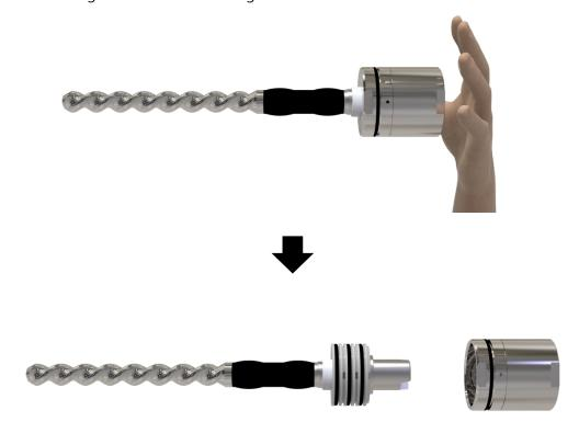
4) Separate the rotary seal and seal support in the rotor direction
