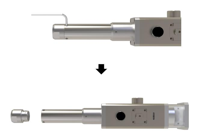
4) Turn the four wrench bolts (M4x10) counterclockwise to separate the stator cap and stator sleeve.
