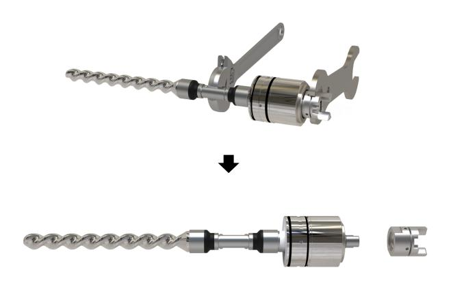
3) Separate bearing block and seal block.
