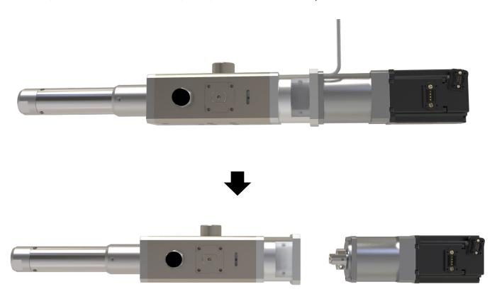
3) Turn the bolts(M3x5) counterclockwise to separate outlet adapter.
