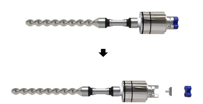
2) Using two spanners, one holds and fixes the D-Cut part of the rotor assembly's rod. Hold the idle coupling with the remaining spanner and turn it counterclockwise to remove it.
