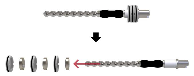
\* Assemble in the reverse order of disassembly.
