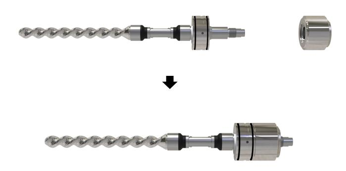
5) Tighten the idle coupling to the end. At this time, make sure that the tee key homes match.
